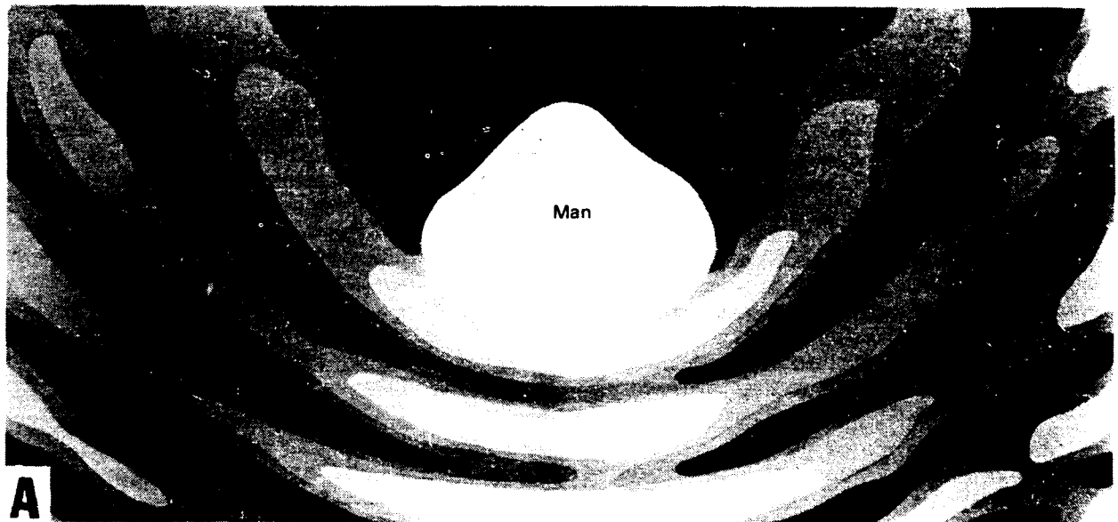
Figure 3-4. Energy distribution in proximity to man at 1 GHz at the chest plane contour presentation; A) vertical, B) horizontal (Reno 1974).
